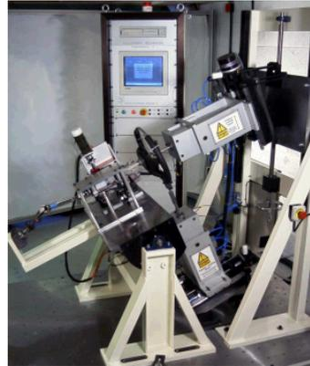
Steering column test rig
