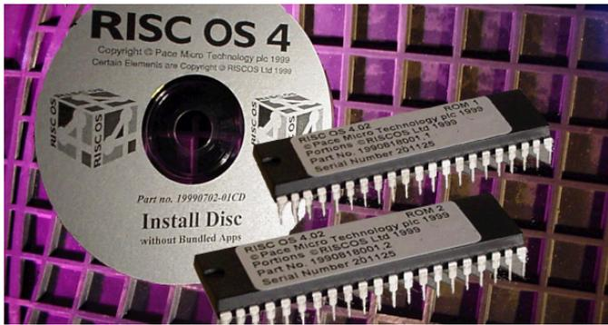
RISC OS is a compact ROM based Operating System solely for use with ARM® 32 bit processors.
